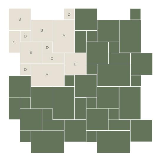
An opus pattern is available in a select few of our natural stone ranges. An Opus pattern is made up of four tile sizes.
